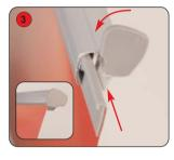
Slide the rail insert and graphic into the top rail. Close the rail end cap.
