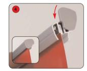
Adhere the flat bar to the **back** of the graphic. Slide the flat bar and graphic into the top rail. Tighten the screws to secure the top rail. Close the rail end cap.
