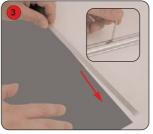
Adhere the flat bar to the back of the graphic. Slide the flat bar and graphic into the top rail. Tighten the screws to secure the top rail. Close the rail end cap.
