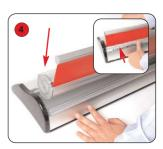
Load the cassette into the base and close the snap retainer to secure. **CAUTION:** ensure fingers are clear of the snap retainer when closing.
